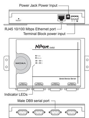
**Reset Button**—Press the *Reset button* continuously for 5 sec to load *factory defaults*: Use a pointed object, such as a straightened paper clip or toothpick, to press the reset button. This will cause the Ready LED to blink on and off. The factory defaults will be loaded once the Ready LED stops blinking (after about 5 seconds). At this point, you should release the reset button.
