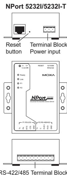
**Reset Button**—Press the *Reset button* continuously for 5 sec to load *factory defaults*: Use a pointed object, such as a straightened paper clip or toothpick, to press the reset button. This will cause the Ready LED to blink on and off. The factory defaults will be loaded once the Ready LED stops blinking (after about 5 seconds). At this point, you should release the reset button.
